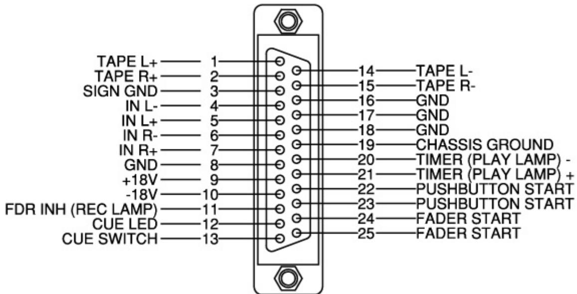
Universal Machine Connection (UMC) for the Eela Audio SBM90 mixing console.
